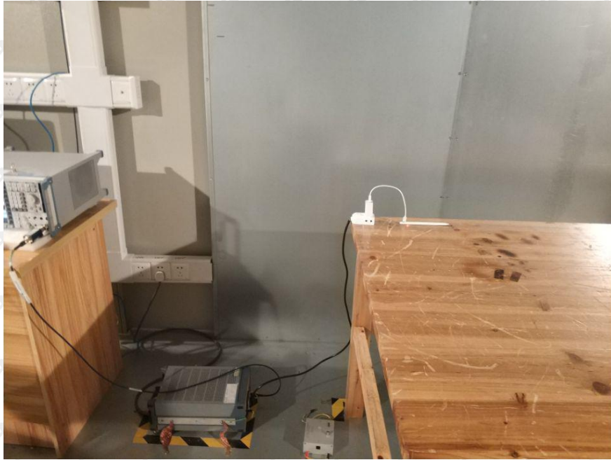
Photograph of test setup for Conducted Emission
